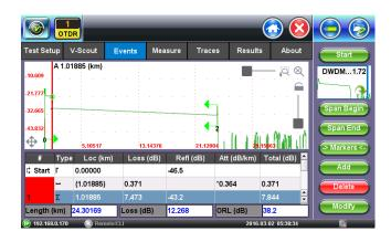
The unit employs specialized software algorithms developed from decades of experience to measure fiber attenuation including anomalies such as connectors, splices, and macrobends.
