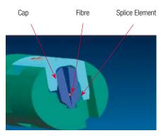
**Cross-sectional view of actuated splice:** After the fibre is inserted, the assembly tool depresses the cap to force clamping and locating surfaces against the fibre, looking and aligning the fibre place.
