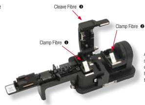
After stripping the coating and cleaning the glass, secure the fibre with the two clamps and activate the cleaver in one step by pressing the lever. The fibre holder maintains the angle orientation from the cleaver to the connector in the assembly tool.
